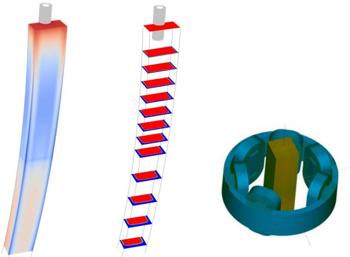
Fig. 1: Example of 3D casting simulation for the new KN3 continuous caster. Left: Temperature field on the billet surface. Centre: Cladding growth dynamics on different spots of the billet. Right: Geometry and Computational mesh of the electromagnetic mixer.
