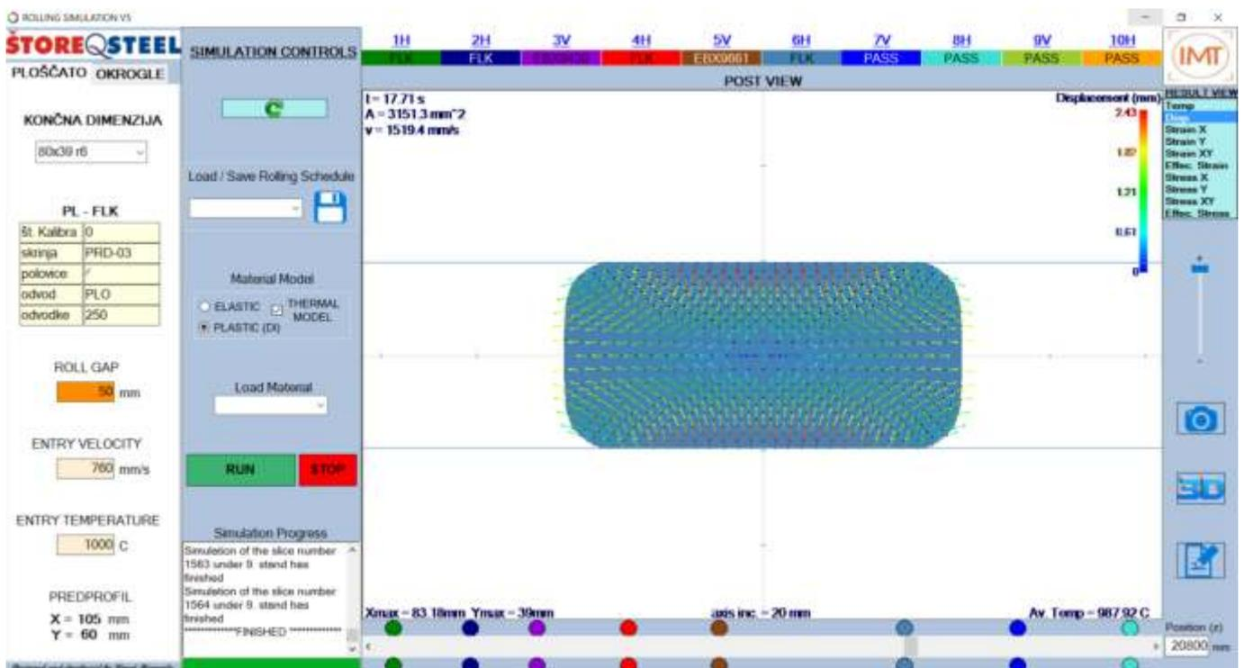
Fig. 3: Graphical interface and simulation example of flat profile rolling.
