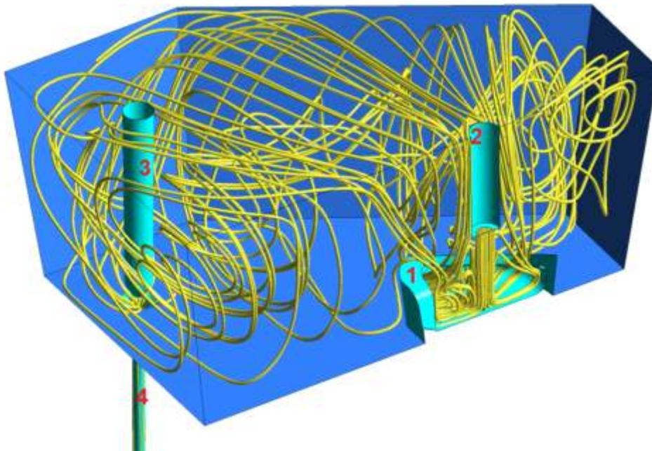
Fig. 2: Calculation result of steel flow in the KN3 tundish with an impact trough "prototype 4". The geometry of the tundish includes: 1-impact trough, 2-shroud, 3-monoblock in 4-discharge. The yellow line presents calculated flow line of steel.
