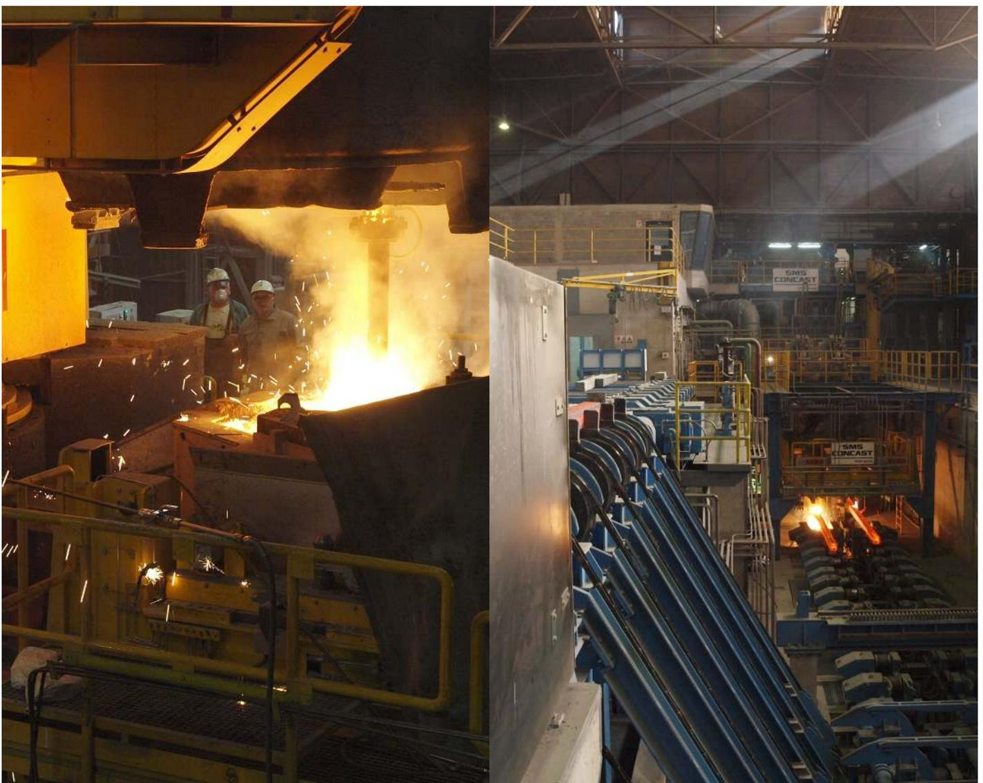
Photo - left: casting platform; photo - right: lower part of the continuous caster
